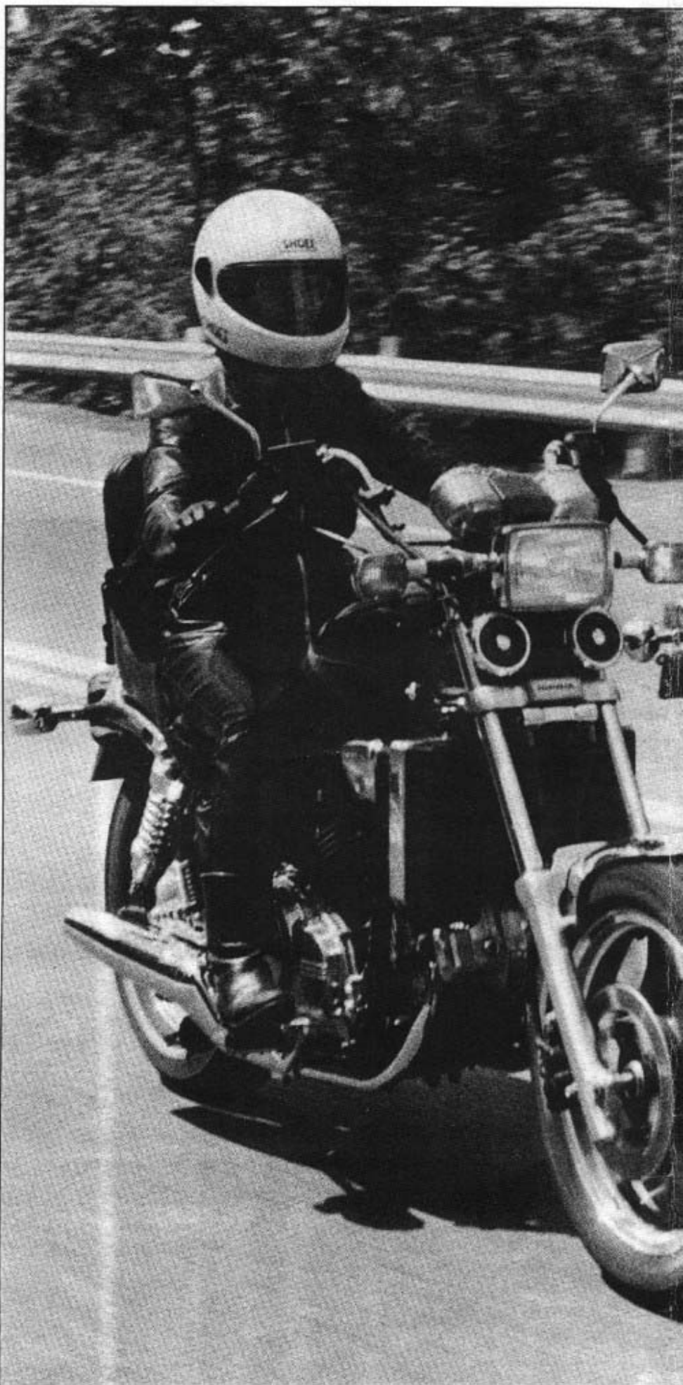
Maxim's disc-type cast rear wheel looks trick but adds unsprung weight.
