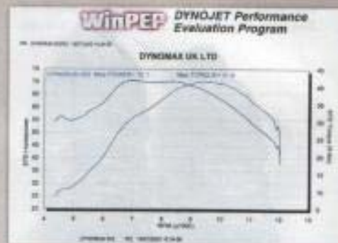
The dyno print out from Dynamax in Horncastle showing the all-important torque curve.
