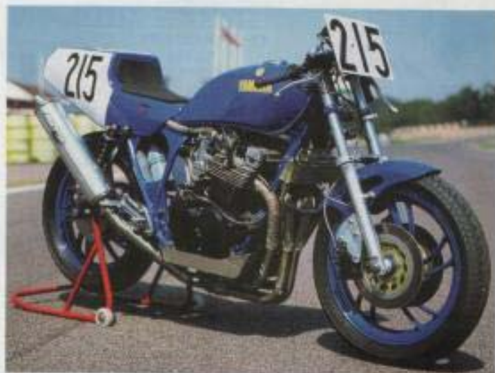
Later FZ600 Yamaha parts have been fitted including the cylinder head.
