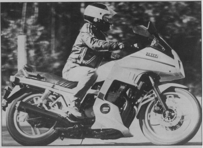
increase in fork rake and trail. New cast wheels with four pairs of parallel spokes replace the curved spoke jobs used on the XJ650.
