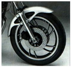
Anatomy of a fixed-up front end: New tire, drilled discs, better brake pads, steel-braided lines and a fork brace. Fork tubes were polished to get rid of pitting and discoloration in the original clear-coat.
