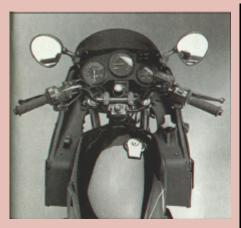
The pilot's view of thr Turbo's cockpit features an FZ750 instrument panel. Note turboboost gauge partially hidden by ignition switch.
