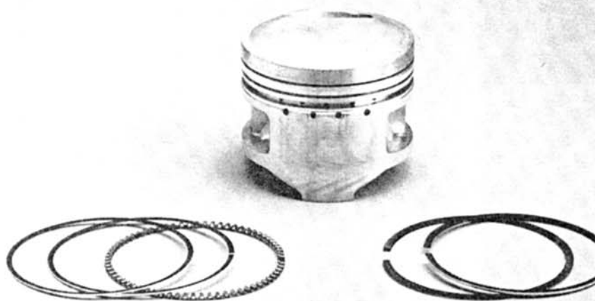
The heart of the project: 68mm Yoshimura cast pistons replaced the stock 63mm pistons, boosting displacement to 761cc.
