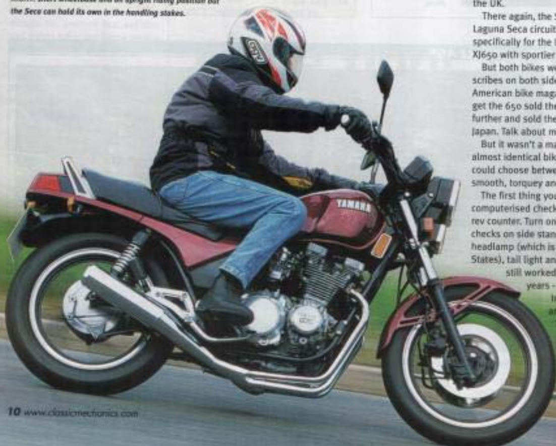
Basically an enlarged XJ650 four cylinder engine.
