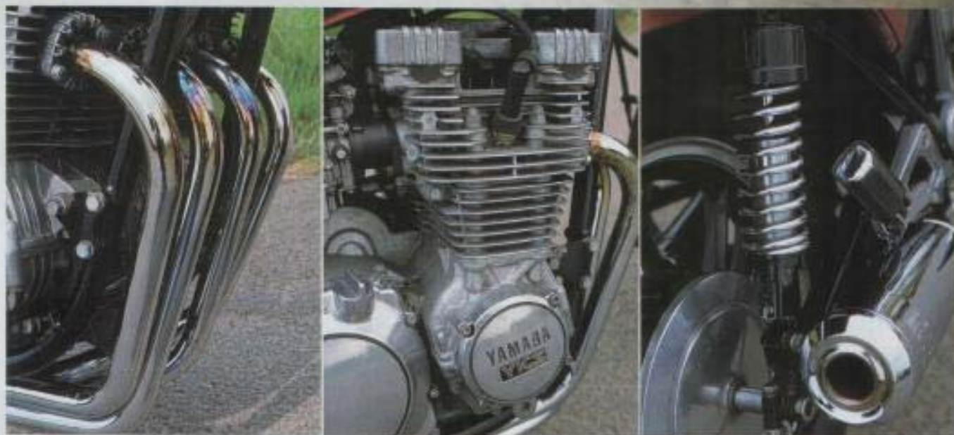
LEFT TO RIGHT: oblique four into one aftermarket exhaust; two valves per each of the four cylinders; multi-adjustable rear shock absorbers.
