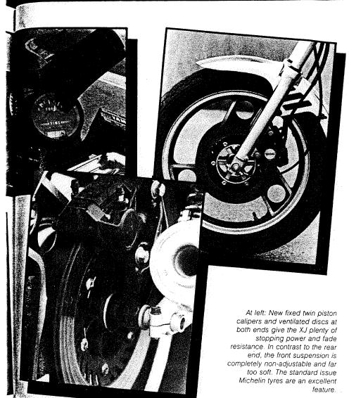
of the areas in which racing technology has been applied to the road, resulting in fixed twin-piston calipers being fitted to the discs on the XJ900, and now the 750. These provide greater power and feel than the old floating piston calipers and when coupled to the XJ's ventilated discs front and rear give a system with excellent fade resistance and fine wet-weather performance.
