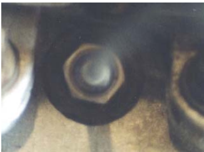
Lean mixture. The flame is a whiteish or electric blue, very hard to see and may disappear completely as the engine "misses".
