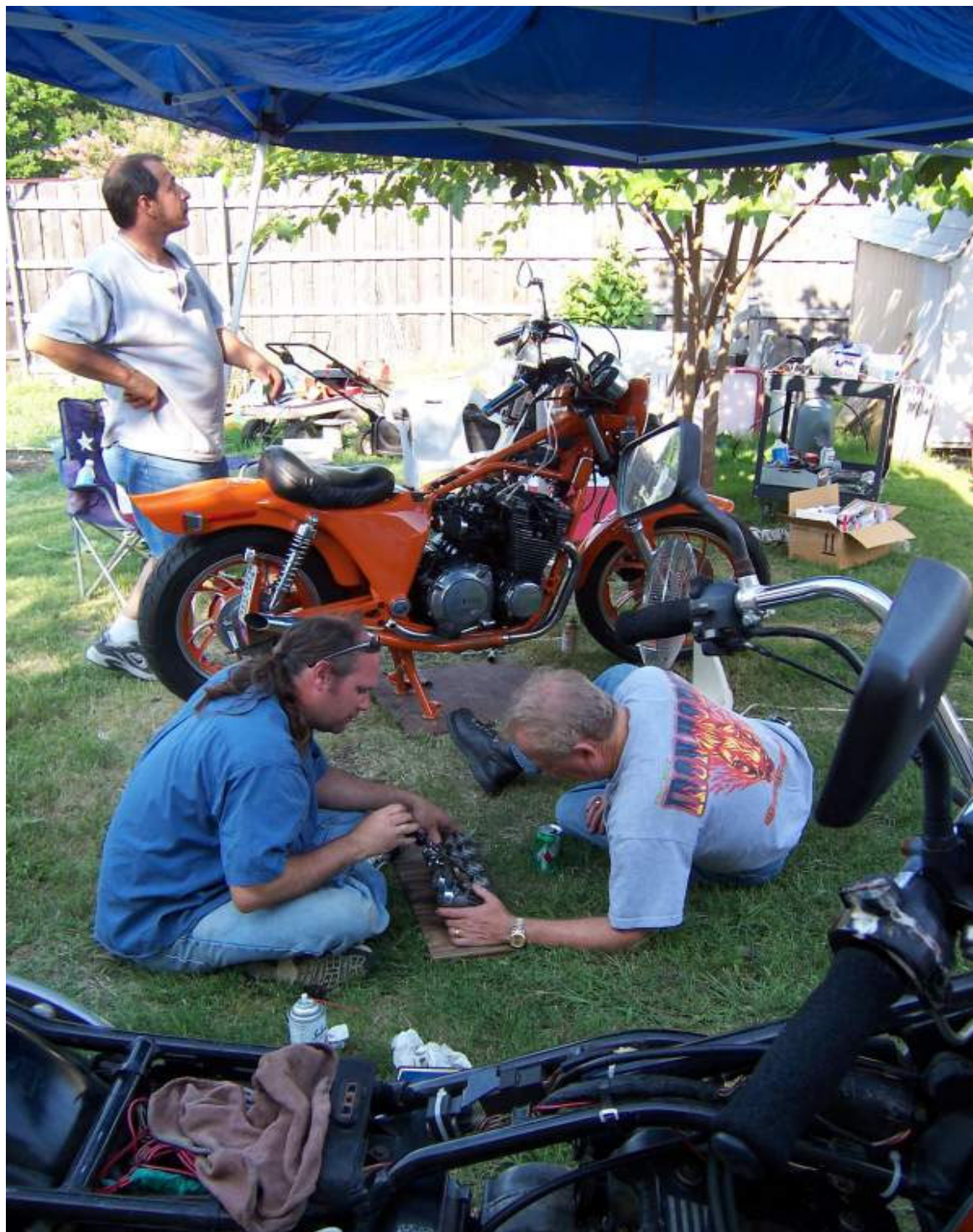
Pulled the Carbs & Adjusted Butterfly Valves : Rex + Carbs
