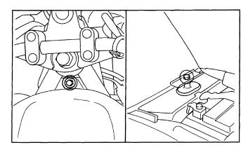
5. Remove the air filter case cover by removing the screws.
