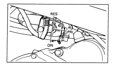
PRI: This stands for "prime". If the engine has been allowed to run out of fuel, turn the lever to the "PRI" position to send fuel directly to the carburetors. This will make starting easier. However, be sure to turn the lever to the "ON" position (or "RES" if you have not refuelled yet) after the engine has started.
