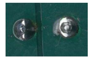
On the left is a good joint. It is bright and shiny and smooth. On the right is the curse of any circuit, a dry joint, note the obvious ring around the wire, this is in fact a crack in the solder caused by either vibration or electrical loading resulting in heat. You can also make out the satin finish on the solder as apposed to the bright smooth appearance on the good joint on the left.
