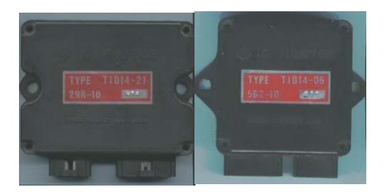
Later type from a 1983 XJ750EII Older type as used on my 1985 XJ750P (Remember the XJ750P is actually based on the 1981-82 Seca and was used as a way to get rid of new old stock parts)
