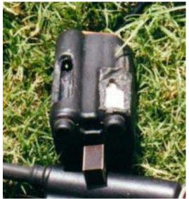
10. Looking from the high tension wire end, you can see that the left side of the coil is the same as the older coils but the other side is very different. The right side wire repair will be described separately and will be referred to as the "right side wire".
