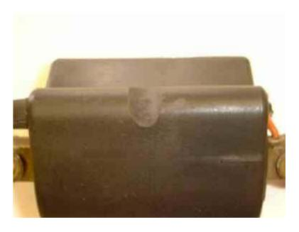
This grind should continue along the length of the coil between the marks. Then, widen the opening to expose more of the wire insulation. See diagram.
