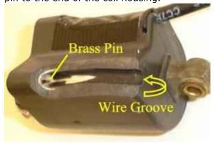
This made it very easy to remove and replace the wires. However, it required cross-drilling the end of the coil in order to secure the loose end of the wires with small zip ties.
