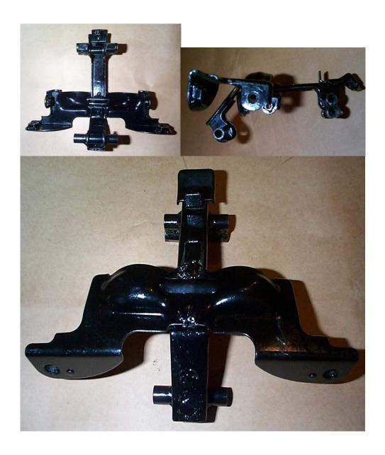
I would now offer everything up to the bike again, recheck, and do any adjustments necessary. You may find the tail touches the bottom of the thermostat. Mine just cleared. If it does mark it, with the coils on, remove it all and put a bend where you marked. Do this with the coils in the cradle so you do not put the coil mount points out of line.
