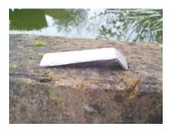
Offer up the ½" end of the bar to the butterfly underneath. The fold on the bar lines with the rear of the butterfly. Line it up as to continue the straight centre line of the bar and weld through the hole you made on the butterfly into the ½" section of bar. The long section should face down to the engine. \* See completed bracket pics \*
