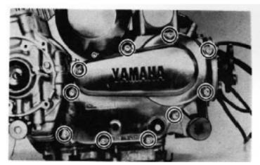
Remove shift lever assembly. Details vary between Seca and Maxim models. Remove cover bolts (circled).
