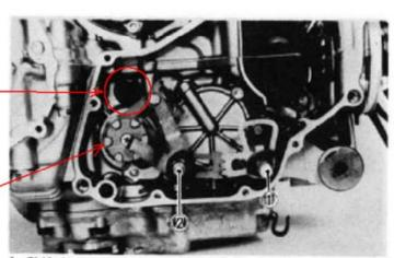
1. Shift lever assembly 2. Shift shaft assembly
