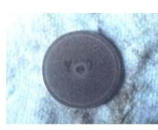
The thickness of the shim is encoded on the back. For example, this once read "Y270", meaning it was 2.70mm thick. The "Y" is also important -- it means the diameter is correct for a Yamaha XJ model. I was once given shims without the "Y" and told (by the service manager) that they were just aftermarket shims. Actually, they were Suzuki shims, and didn't fit properly!
