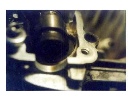
Before installing the valve shim tool, rotate the engine so the cam lobe pushes the shim and bucket down fully.
