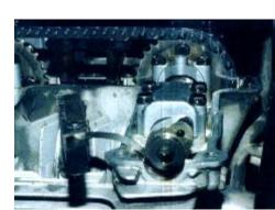
With the engine cold, remove the valve cover. Using feeler gauges, measure and record the clearance of each valve with the lobe opposite the shim and bucket. The feeler gauge should slide in and out easily, with a slight resistance.
