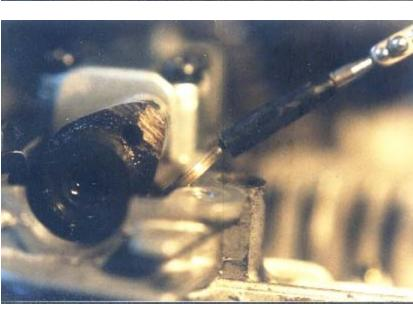
A magnet, tweezers or small needlenose pliers will be required to extract the shim from between the camshaft and the bucket.
