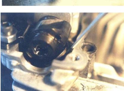
Once the tool is in place, rotate the engine so the camshaft lobe rotates away from the tool. This is important! Rotating the camshaft lobe toward the tool will cause damage! The bucket and shim should be held down by the tool as the lobe is rotated away, allowing the shim to be popped out of the bucket with a thin screwdriver.
