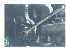
Rotate the engine as required by using a wrench on the ignition rotor. Check the clearance against the specifications for your machine. If any are out of range, they must be changed. Remember that most machines have a different specification for exhaust and intake valves. This is because the exhaust valves run hotter and expand more.
