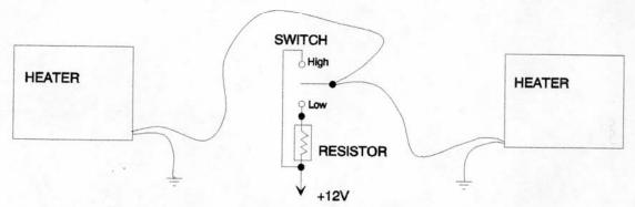
OPTION 1, Using supplied switch and resistor. Advantage: simple and all parts supplied in kit.
