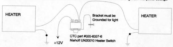
OPTION 3, Buy new rotary switch. Advantage: 4 position (Off, High, Med, Low) and built in resistor. Illuminated knob for night use. Comes with bracket (may not need project box). Very simple to wire.
