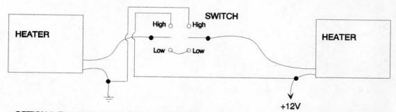
OPTION 2, Buy new DPDT switch and delete resistor. Advantage: less power use on Low setting.
