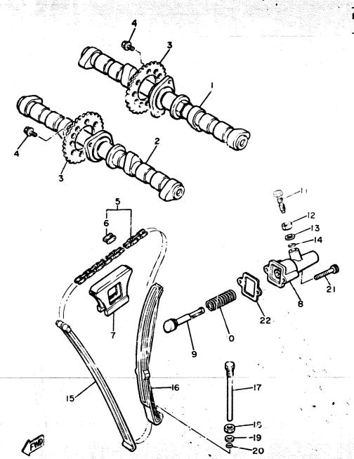
FIG. 4 CAMSHAFT-CHAIN
