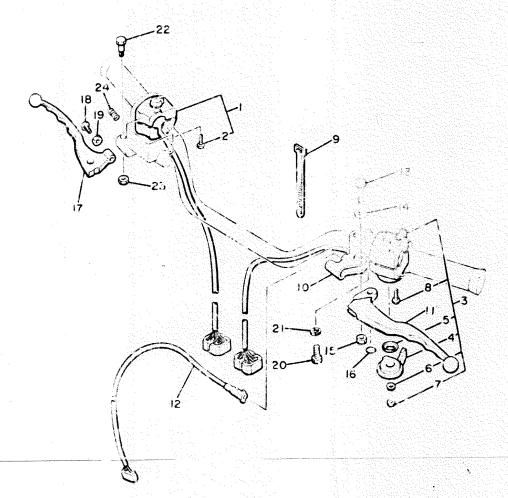
FIG. 45 HANDLE SWITCH LEVER
