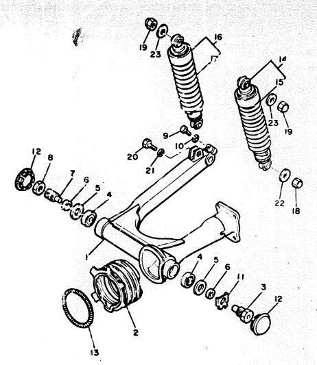
FIG. 27 REAR ARM. SUSPENSION
