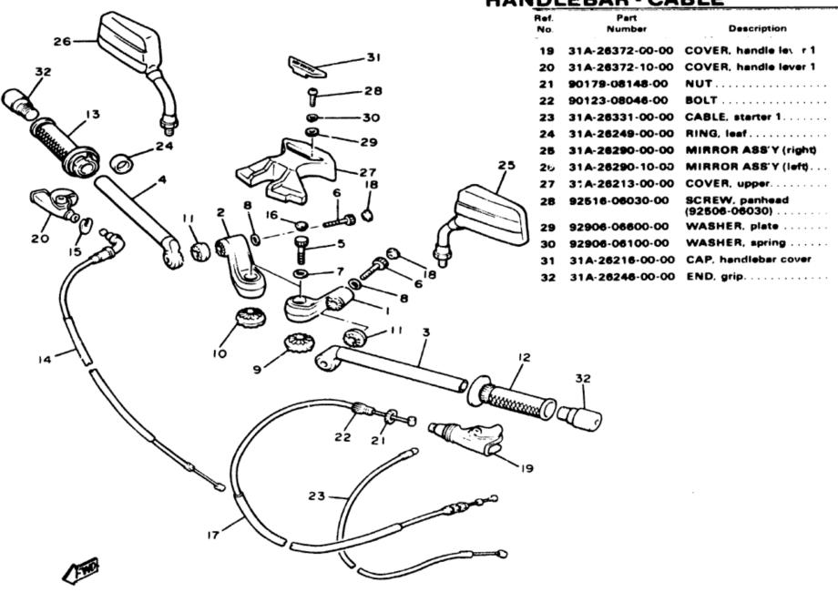
FIG. 33 STEERING HANDLE. CABLE
