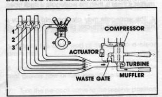
Exhaust (or turbocharger) and lubrication problems usually fall into two categories: oil leakage from the exhaust and lack of lubrication at the turbocharger.
