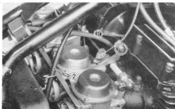
1. Starter (CHOKE) cable 2. Clutch cable
