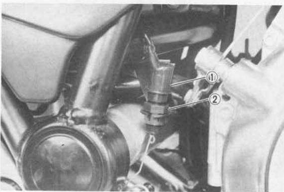
1. Main body 2. Adjusting nut
